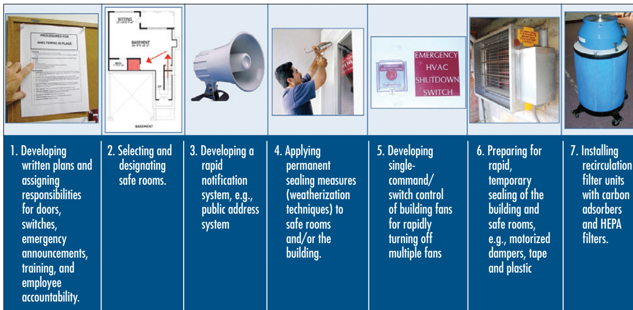
Figure 5-2: Setting up a safe room
